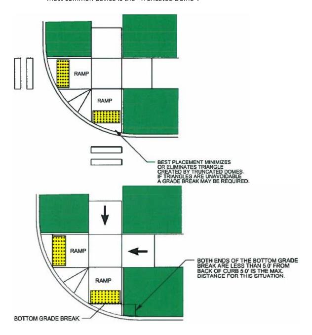
Figure 7: Detectable Warning Devices
