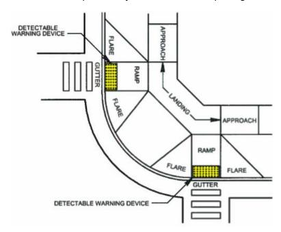
Figure 6: Standard Perpendicular Curb Ramp Components
