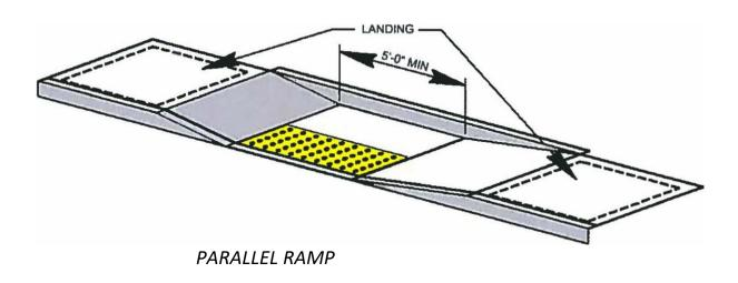
Figure 11: Parallel Curb Ramp
