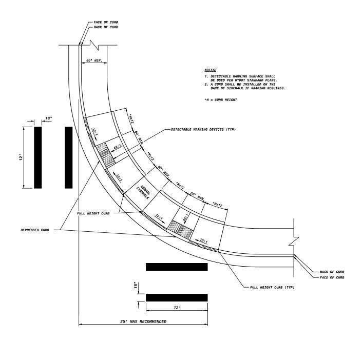
APPLICATION FOR THIS DETAIL IS APPLIED TO URBAN OR SUBURBAN INTERSECTIONS WITH LARGE CURB RADII AND NARROW SIDEWALKS. IT DOES NOT ALLOW FOR PEDESTRIANS TO ENTER AN INTERSECTION AND CROSSWALK AT A RIGHT ANGLE. USE OF THIS DETAIL IS MOST APPROPRIATE AT SIGNALIZED INSTERSECTIONS. SINCE THE SETBACK OF THE RAMP FROM THE CROSSING ROADWAY REQUIRES THAT THE STOP BAR BE INSTALLED FARTHER BACK THAN IS DESIRABLE FOR SAFE OPERATION AS A STOP-CONTROLLED INTERSECTION.
