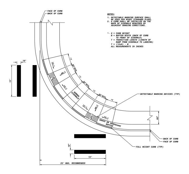
APPLICATION FOR THIS DETAIL IS APPLIED TO INTERSECTIONS WITH LARGE CURB RADII AND NARROW SIDEWALKS. IT DOES NOT ALLOW FOR PEDESTRIANS TO ENTER AN INTERSECTION AND CROSSWALK AT A RIGHT ANGLE.
