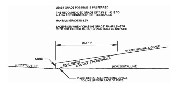
Figure 26: Curb Ramp Grade Retrofit
