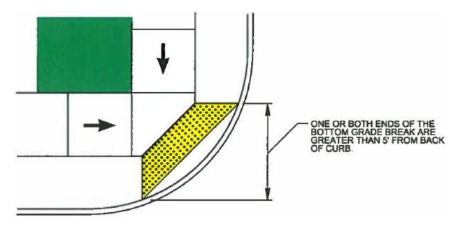
Figure 7 (Cont.): Detectable Warning Devices
