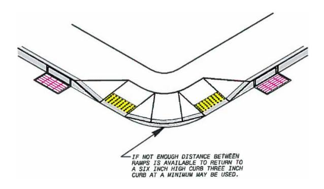
Figure 32: Lower Curb Between Ramps
