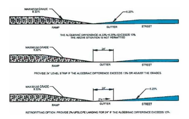
Figure 16: Counter Slope
