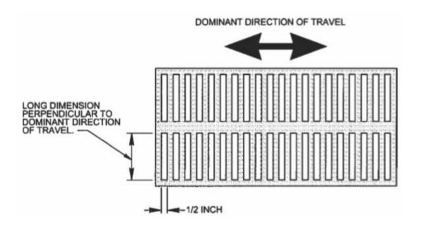
Figure 3: Horizontal Openings
