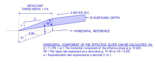
RESULTANT TAPER WIDTH = SURFACING DEPTH X 1:5 TAPER SLOPE = 1ft X 5 = 5 ft. TAPER WIDTHS ARE FIXED AND DO NOT CHANGE WITH SUPERELEVATION ROTATION TAPER SLOPES ARE RELATIVE TO THE PAVEMENT TOP AND ROTATE WITH SUPERELEVATION.
