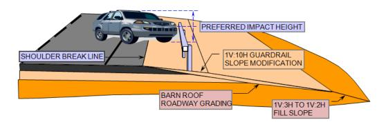
**EXHIBIT 13** GUARDRAIL WITH 1V:10H SLOPE MODIFICATION
