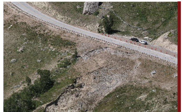
Point cloud of the Little Tongue River slide. A point cloud is a 3D model of millions of individual georeferenced photography and ground control points.
