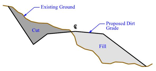
Figure F-11. Cross-section with cut and fill areas.
