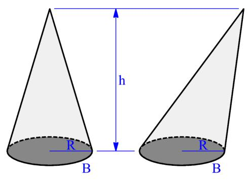
Figure F-7. A right cone and an oblique cone.
