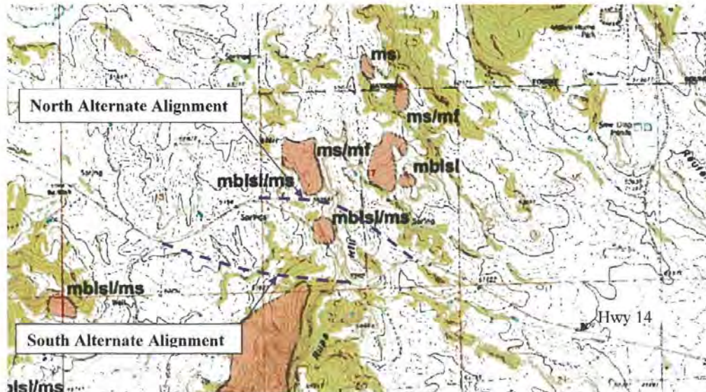
Figure 1: Wyoming State Geological Survey Hazard Map for Highway 14 west of Sundance. Rupe Hill is mapped as a multiple block slide/multiple slide (mbisl/ms) complex. Two alternate alignments were considered to avoid the landslide; a south alignment and a north alignment.
