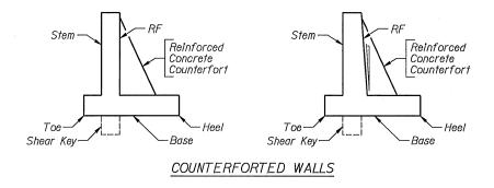
**EXPANSION JOINTS** and **CONTRACTION JOINTS** may be required for cantilever and counterforted walls. Expansion joints shall be provided if the wall length exceeds 90'-0". Contraction joints shall be provided at spacings of 20'-0" minimum to 30'-0" maximum.
