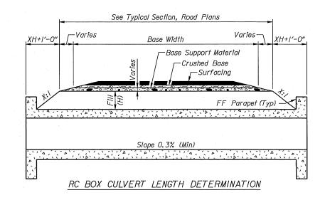
The **SIZE** of a culvert used as a hydraulic structure is based on the Hydraulic Report, which provides several alternates of opening sizes and depths of cutoff walls. The Squad Team Leader will select one of the sizes recommended and include it in a Structure Selection Report.
