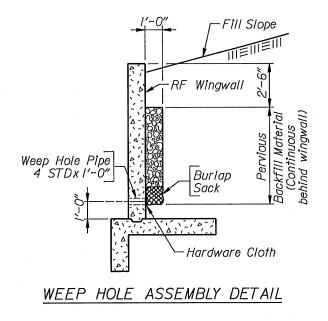
Each weep hole assembly consists of a pipe 4 STD through the wingwall, one  $6'' \times 6''$  piece of aluminum or galvanized steel wire 4 mesh hardware cloth (Minimum wire diameter 0.03'') centered over pipe end and firmly anchored to rear face of wingwall, and one cubic foot of coarse aggregate in a securely tied burlap sack.
