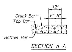
4.13 - 3 Apr 2007 Rev Nov 2018 For slabs that have **SKEWS LESS THAN OR EQUAL TO 20 DEGREES**, the transverse reinforcing steel shall be placed parallel with the substructure and dimensioned along the edge of the slab. Consideration should be given to placing this reinforcing steel parallel with the substructure on bridges of any skew with composite girders due to possible clearance problems with the shear connectors.
