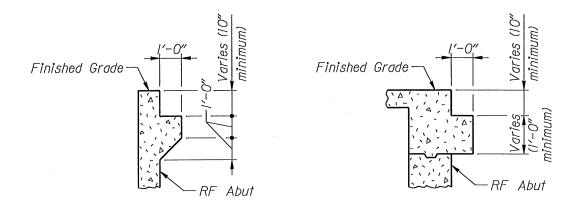
**SEAT SIZE** shall be of sufficient dimension to minimize the chance of concrete spalling when the loads are placed. As a general guideline, the sketch below should be used for typical situations and adapted to suit other situations as well.
